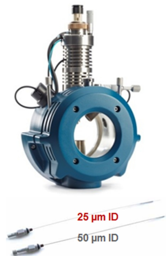
Figure 2: IonDrive™ Turbo V Source. The optimized geometry and larger diameter heaters provide more efficient heat transfer to a larger cross section of the spray cone. Equipped with the lower inner diameter hybrid electrodes from Eksigent, this source provides a robust easy to optimize solution for microflow chromatography.
