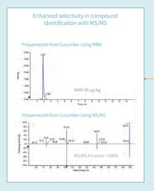
QTRAP technology enables collection of high-quality MS/MS spectra in addition to MRMs to enable library comparisons for better confidence in compound identification.
