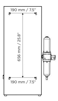
The generator can be wall mounted, **If do not wish to wall mount your generator** proceed to step 4.
