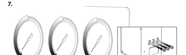
The purge is now complete. Disconnect the air supply then, once the pressure gauges on the front of the generator read 0, the **silencer fittings can be removed** from the Curtain, Source & Exhaust ports.
