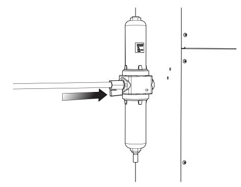
Attach your house air supply to the **BA filter** at the **left side** of the generator. Ensure the valve on the filter is at the **open** position.
