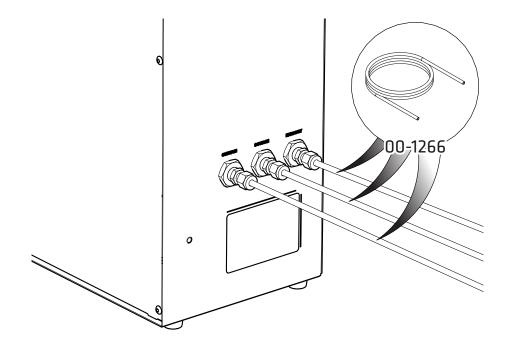
Select the supplied 1/4" PTFE Tubing 00-1266 and connect this to the three 1/4" x 1/4" Compression Fittings 02-4421.
