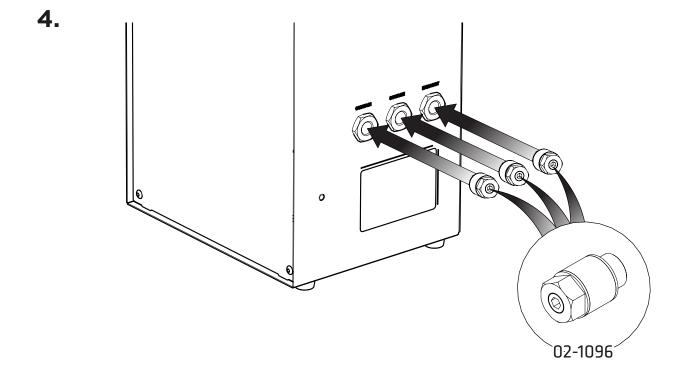
Select the **3** × **02-1096 Flow Control Silencer** and attach them to the **Curtain, Source** & **Exhaust** outlets at the right side of the generator.
