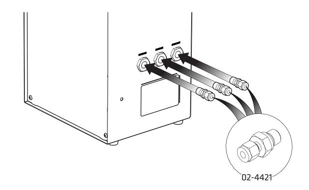
Select the **3** × **1/4**" **Compression Fittings 02-4421** and attach them to the **Curtain, Source** & **Exhaust** outlets at the right side of the generator.
