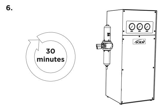
Leave the generator **connected to your air supply** for a period of **30 minutes** to purge the system.
