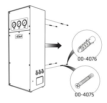
With the holes drilled in your desired location, fit the  $4 \times No. 8$  Wall Plug 00-4076 and  $4 \times No. 8$  Screw 00-4075 to the wall and mount your generator onto them.
