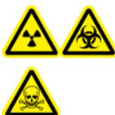
**WARNING! Ionizing Radiation Hazard, Biohazard, or Toxic Chemical Hazard.** Vent the source exhaust system to either a dedicated laboratory fume hood or an external ventilation system to prevent hazardous vapors from being released in the laboratory environment.
