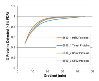
**Figure 6. Selecting the Best Chromatographic Strategy.** Plotting the proteins identified relative to the numbers obtained on the typical longer 45 min gradient, the resulting decrease in the protein ID numbers is surprising low. Using a 10 minute gradient, about 70% of the proteins are still identified, and even at 5 mins, 50% of proteins were still confidently identified relative to the longer gradient.
