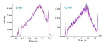
Figure 2. High Gradient Reproducibility. Even for that fastest gradients, very reproducible ion chromatograms were observed. TOF MS TICs for the 5 and 10 minute gradients are shown.
