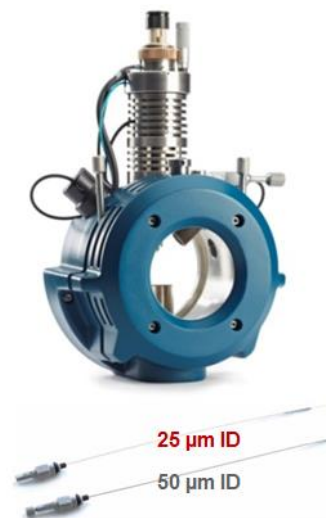
Figure 2: IonDrive™ Turbo V Source. The optimized geometry and larger diameter heaters provide more efficient heat transfer to a larger cross section of the spray cone. Equipped with the lower inner diameter hybrid electrodes from SCIEX, this source provides a robust easy to optimize solution for microflow chromatography.
