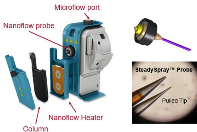
Figure 6. OptiFlow Source Configuration for Nanoflow LC-MS. Nanoflow probe and electrode are installed in the port on the front of the source and the microflow port is closed with the plug. The nanoflow column heater mounts on the front of the source and cartridge based nanoflow columns from Phenomenex can be inserted easily. (Right top) The nanoflow probe is pre-configured so the probe/electrode mount the same with the same protrusion every time. Nebulizing gas flows coaxial to the electrode. (Right bottom) Nano electrodes are designed for robustness, produced by grinding the outside of tip to produce a taper. This ensures no internal constriction at the end and reduced chance of plugging compared to a pulled tip design.
